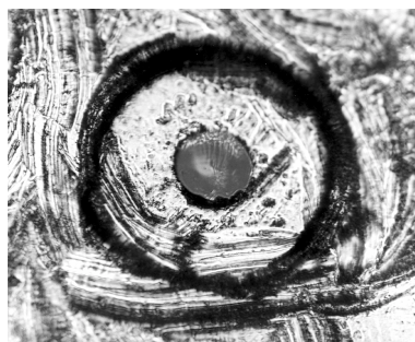
Figure 1-6. Damage from improper cleaning.
